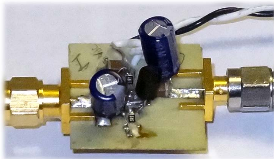
Figure 39 : Transimpedance amplifier circuit to convert the photodiode current to a measurable voltage.
