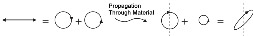
Figure 13 : Illustration of the Faraday ellipticity mechanism.
