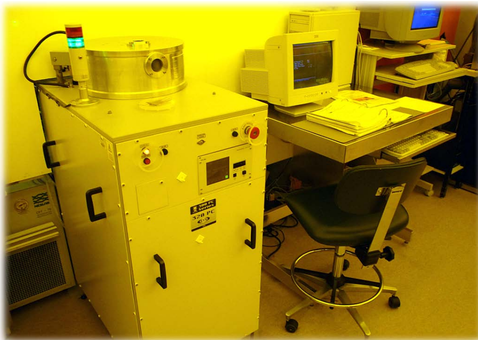
Figure 98 : STS Model 320 reactive-ion etching system.
